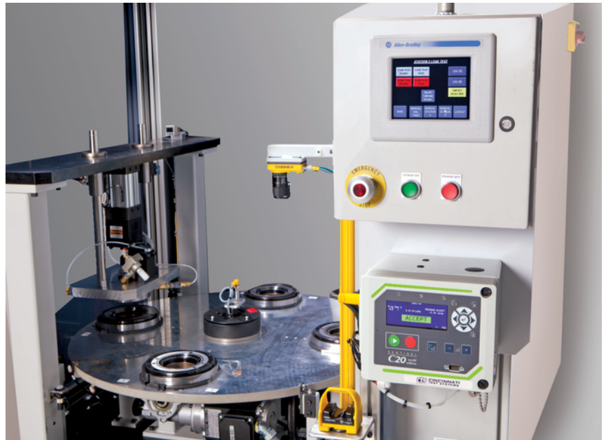
C20 integrated into an automated test cell
